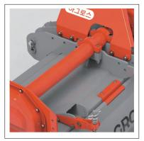
• Main deck with frame structure with high-strength double BEAM
